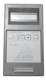
displays the results. It is also equipped with a buzzer and LED which will alert the user as to any suspicious result.
